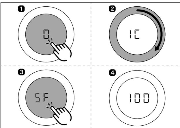
Fig. 5.20 Displaying the remaining filter service life
