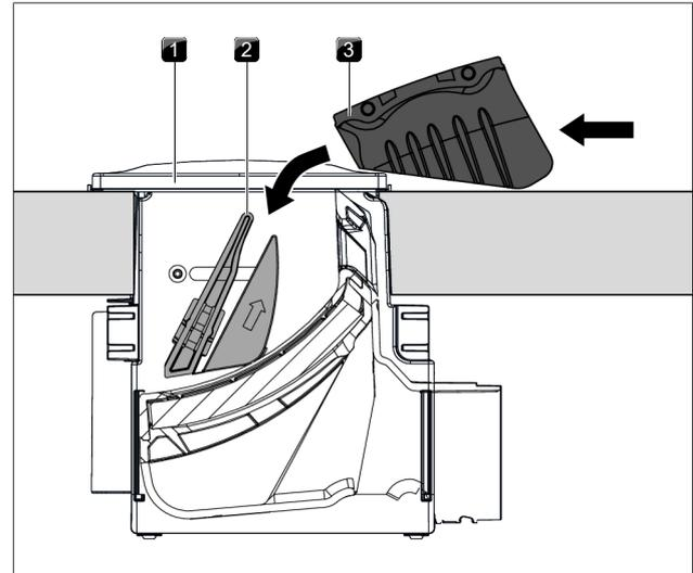
Fig. 7.3 Fitting the cover flap
