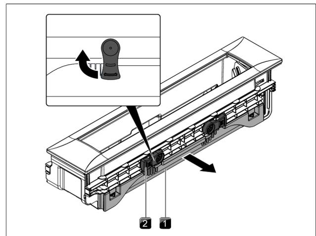
Fig. 7.4 Removing the maintenance tray
