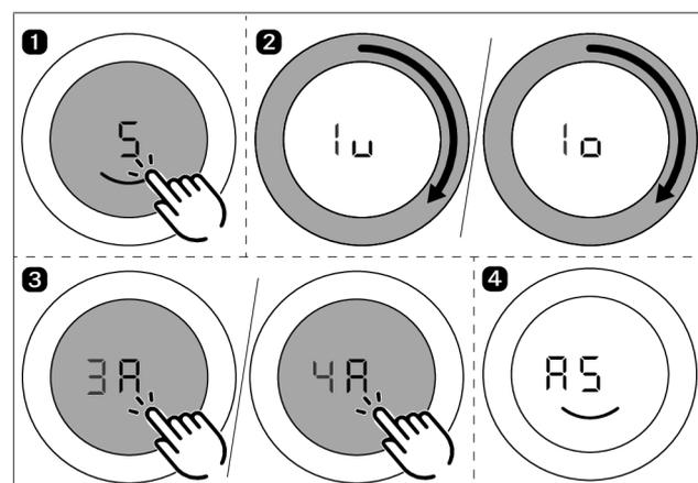
Fig. 5.39 Activating the automatic heat up function
